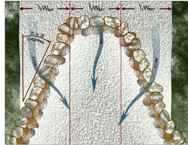
CROSS-VANE STRUCTURE, FROM ROSGEN
